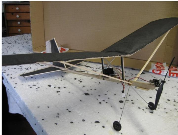
A modified F/F Hanger Rat for indoor RC. Uses an F929 spare part RX/servo (£7.84) an HFW400 spare motor assembly (£3.13) and a 1S 150mah LIPO (£1.76), All available from [www.Banggood.com](http://www.Banggood.com) .I have a WLtoys v911 helicopter and that binds with the F929 RX. A bit of balsa and tissue and a couple of hours work, that's RC on the cheap!
